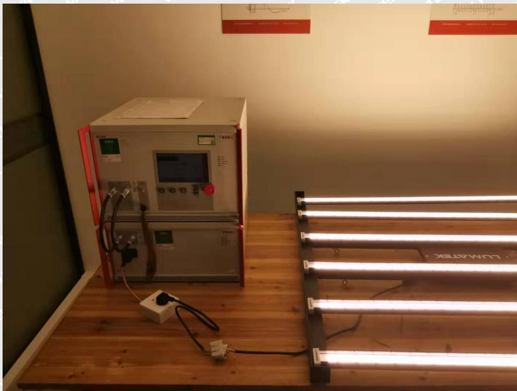
7.9 Photograph – Injected Currents Immunity Test Setup
