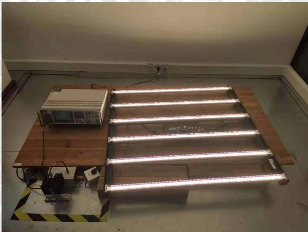
7.9 Photograph – Injected Currents Immunity Test Setup
