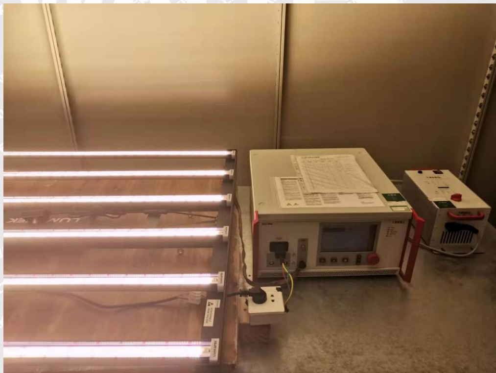
7.8 Photograph – Surge Immunity Test Setup
